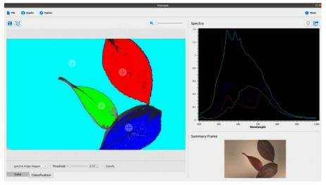
The application software features easy and fast data cube capture and intuitive image classification/segmentation as part of a suite of powerful spectral image exploration tools.
